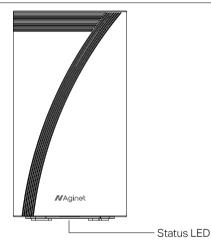
LED Device Status Flashing yellow The device is starting up or resetting. The connection quality of the device is normal. Flashing blue The device is ready for setup. Fast flashing blue The device is establishing a WPS or mesh connection. The device has been set up, but the internet is unavailable. Flashing green The device is upgrading firmware. The device is all set up and connected to internet. Flashing red The device has lost connection. The device has an issue.
